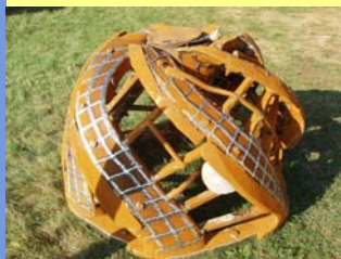
Dredge cutter head used to dislodge lake sediment
