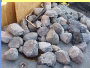
Rocks from lake bottom that entered dredge pump
