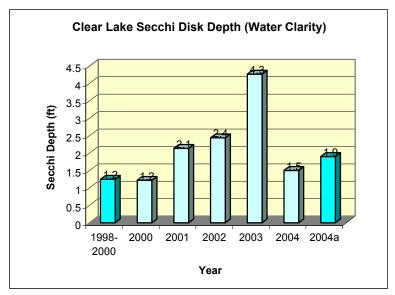
Secchi disk depth is a means of measuring water clarity.
